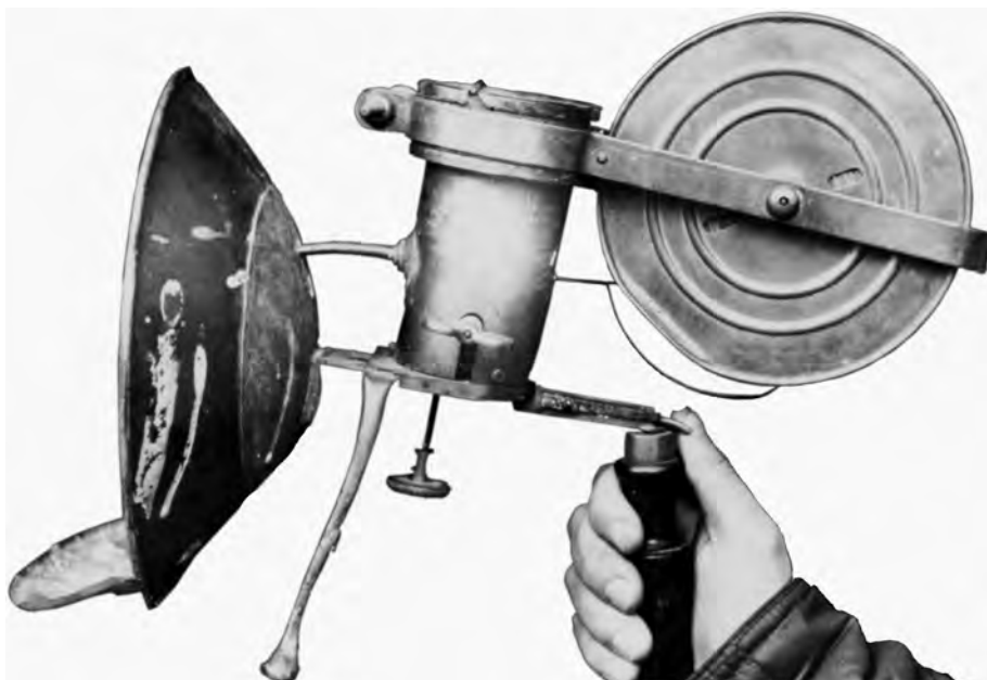
Figure 5 : A magnesium ribbon lamp like that of Louis Armand, with a reflector and a clockwork movement. Photo Jean-Pierre Bonnebouche.
